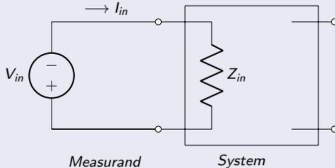
If the measurand is voltage, then  $Z_{in}$  must be large so that very little current is drawn from the measurand and voltage measured by the system is almost equal to  $V_{in}$ .
