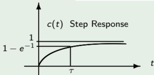
$$\mathcal{L}\{u(t)\} = U(s) = \frac{1}{s} \quad \text{and} \quad \frac{Y(s)}{X(s)} = \frac{1/RC}{1/RC + s} \rightarrow C(s) = H(s)U(s) = \frac{1}{s} \frac{a}{a+s} = \frac{1}{s} - \frac{1}{s+a}$$
