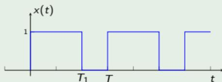
$$\begin{aligned} a_k &= \frac{1}{T} \int_0^{T/2} 1 \cdot e^{-jk\omega_0 t} dt = -\frac{[e^{-jk\omega_0 T/2} - 1]}{Tjk\omega_0} \\ &= e^{-jk\omega_0 T/4} \frac{[e^{jk\omega_0 T/4} - e^{-jk\omega_0 T/4}]}{Tjk\omega_0} \\ &= e^{-jk\pi T/4T} \frac{\sin(k\pi T/4T)}{k\pi} = e^{-jk\pi/4} \frac{T/4}{T} \operatorname{sinc}(k \frac{T/4}{T}) \end{aligned}$$
