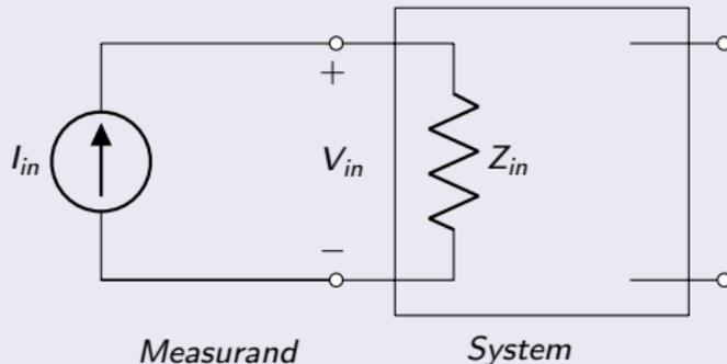
If the measurand is current, then  $Z_{in}$  must be small so that very little voltage is dropped across the measurand and current measured by the system is almost equal to  $I_{in}$ .
