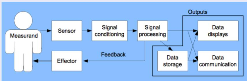
Measurand : Physical quantity, property, or condition that the system measures *biopotential, pressure, flow, dimension (imaging), displacement (velocity, acceleration, and force), impedance, temperature, chemical concentrations.*
