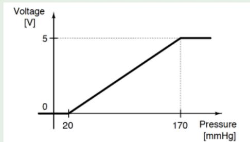
a) Find the sensitivity of the transducer, and the range of pressure over which it operates.
