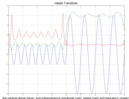
the original signal (blue), and instantaneous amplitude (red), phase (red) and frequency (green)
